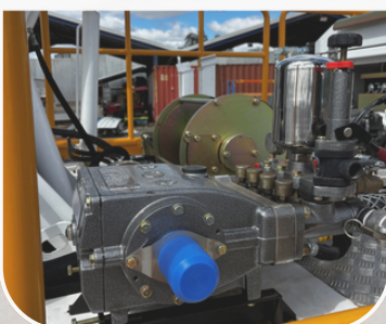
140LPM WATER INJECTION PUMP
